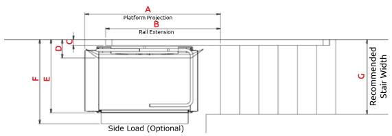
NOTE: Dimension F only applies at lower landing when the side load ramp is in the open position.
