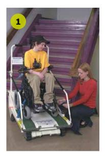
A small operator can easily transport a passenger in a heavy power wheelchair. Above, the passenger has boarded the platform using the integrated ramp. The wheelchair is secured by four adjustable tie-down straps. An electrically interlocked seat belt provides passenger security.
