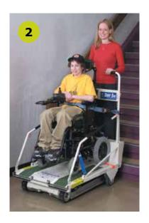
Once the Super-Trac has been rolled to the base of the stairway, the operator will then tilt the platform using the hydraulic tilt control, and begin climbing the stairs.
