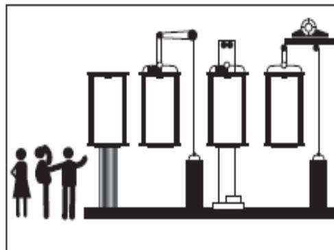
While most home elevators are safe if installed, operated and maintained correctly, there are some home elevator models and features which pose greater risk, especially to children, and should include additional features to enhance safety, including: vanishing elevator models, models with accordion-fold door gates and models with scissor-style gates.
