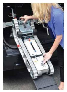
The optional vehicle loading ramp allows the Stair-Trac to be easily and safely loaded and unloaded from vehicles using the drive motor.
