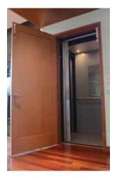
Residential swinging passage doors are supplied by others as hall doors. During the installation of your elevator, the doors are fitted with special interlocks. They will open only when the elevator car is at the same landing. Solid core or solid wood core doors are required. The doors can be equipped with an optional automatic door operator.
